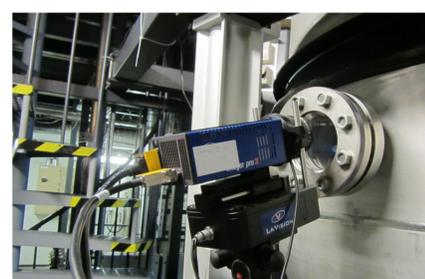
Figure 4. Placement of a camera to the PPOOLEX test facility.
