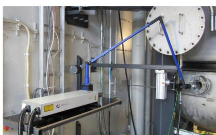
Figure 3. Placement of the laser to the PPOOLEX test facility.
