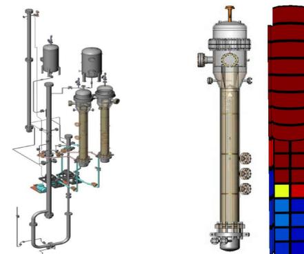
Figure 2. PWR PACTEL facility, vertical steam generator and visualization of calculated void fraction in the steam generator secondary side model.
