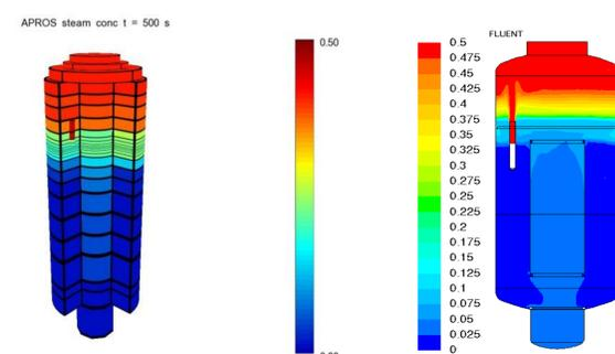
Figure 3. Steam molar fraction at  $t = 500$  s calculated with Apros (left) and Fluent (right) in the THAI TH24 experiment.
