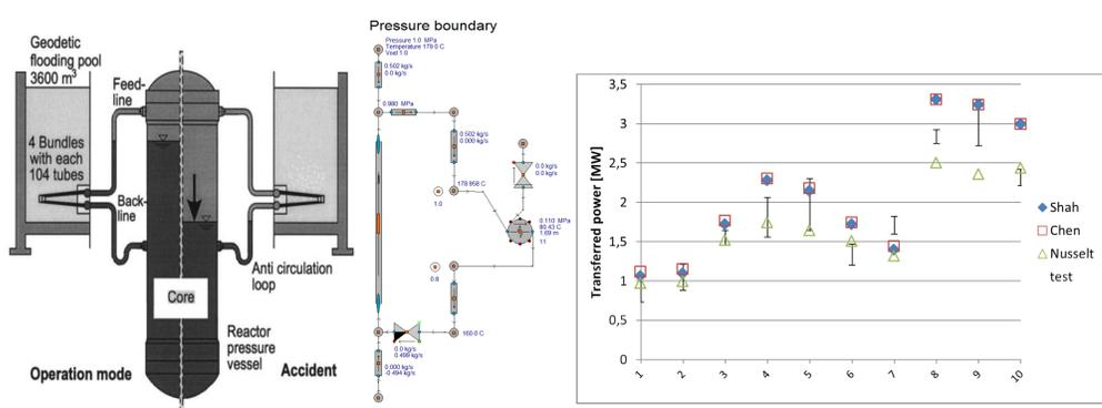
Figure 1. Principle of the emergency condenser, Apros model of the NOKO experiment and calculated heat transfer rate in all the 10 test cases with three different interfacial heat transfer correlations.
